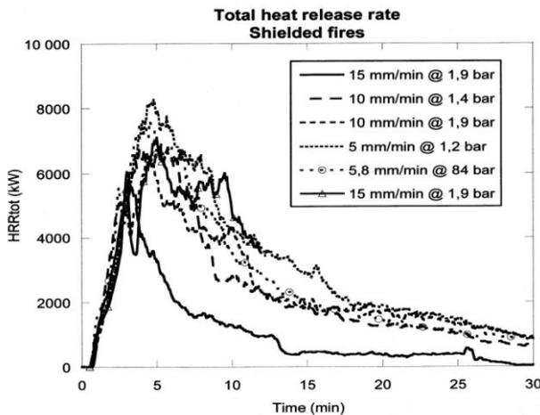
Figure 3: Total heat release rate for shielded fires in full scale test (Arvidson 2010<sup>2</sup>)
