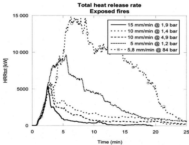
Figure 1: Total heat release rate histories for the fire tests using various water application rates and pressures without shielding. (Arvidson 2010<sup>2</sup>)
