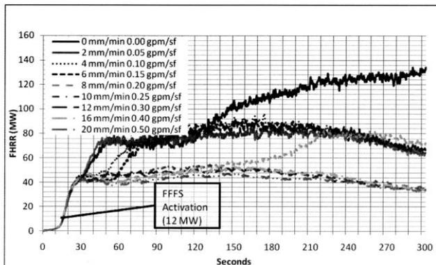
Figure 4: Fire heat release rate for shielded tests using CFD analysis (Harris 2010<sup>6</sup>)
