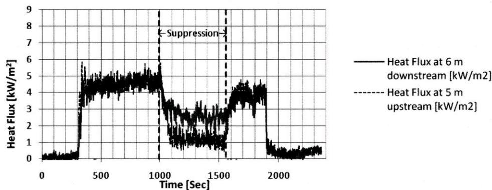
Figure 3: A comparison of heat fluxes measured 5m downstream and 6m upstream over time (Yoon J. Ko and George Hadjisophocleous 2010<sup>7</sup>)
