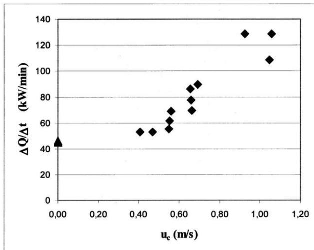
Figure 4: The fire growth rate as a function of the longitudinal ventilation velocity<sup>13, 14</sup>
